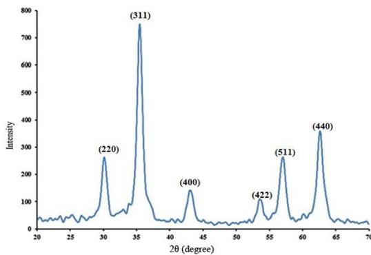
**Figure 1.** XRD patterns of Fe<sub>3</sub>O<sub>4</sub> nanoparticles.
