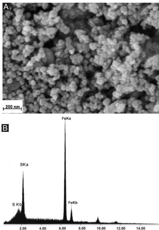
**Figure 2.** (A) SEM image of DNP@SDS@Fe<sub>3</sub>O<sub>4</sub> nanoparticles; (B) SEM-EDX spectrum of SDS@Fe<sub>3</sub>O<sub>4</sub> nanoparticles.
