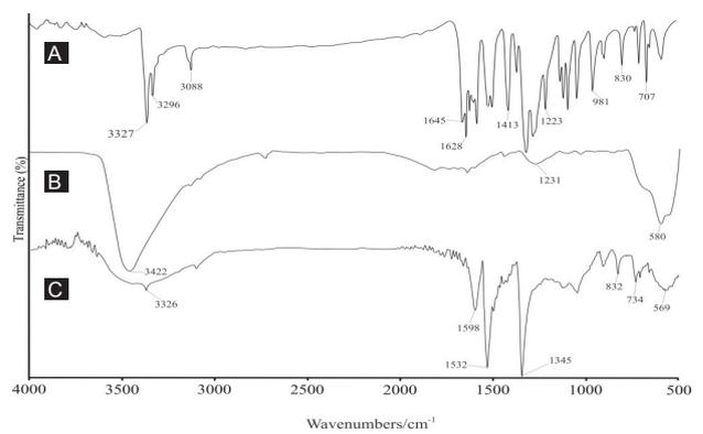
**Figure 3.** FTIR spectrum of: (A) 2,4-DNP; (B) magnetite nanoparticles; (C) DNP@SDS@Fe<sub>3</sub>O<sub>4</sub> nanoparticles
