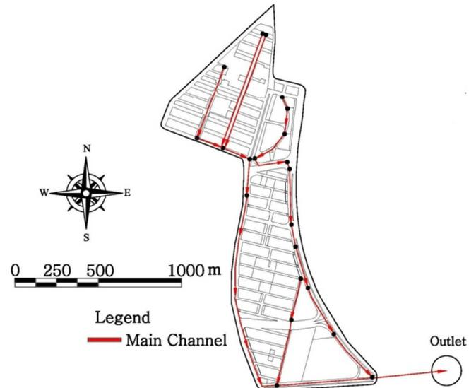
Fig. 3 The layout of main urban drainage channels
