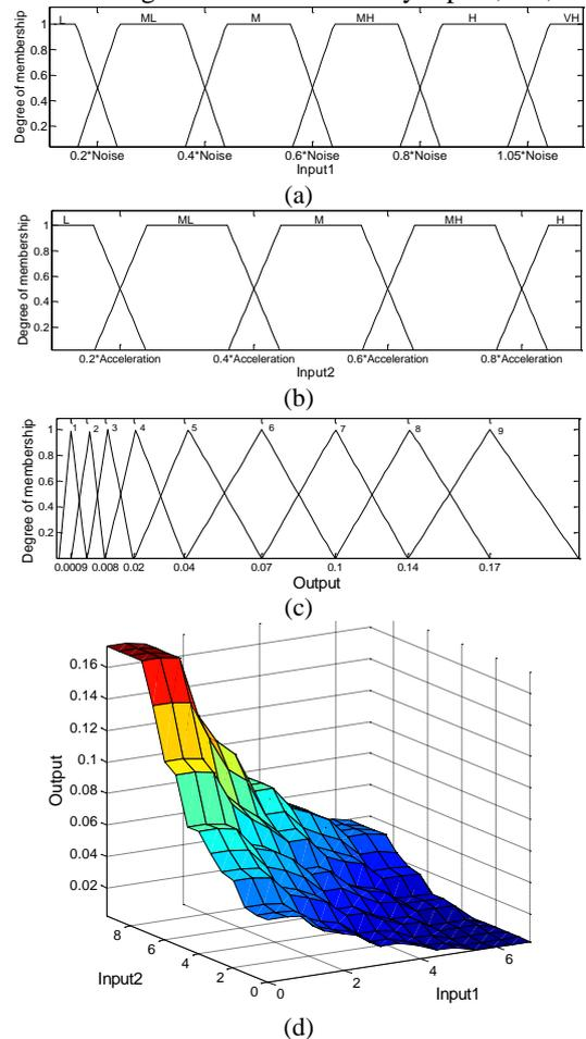
Fig. 6 (a) MFs of fuzzy Input1( $x_1, y_1$ ), (b) MFs of fuzzy Input2( $x_2, y_2$ ) (c) MFs of fuzzy output, (d) Surface of desired outputs.
