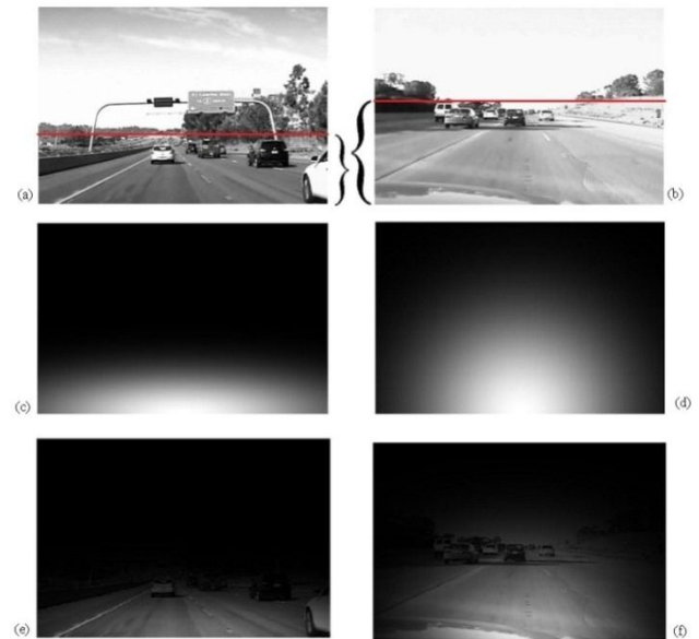
Fig. 3. Angular installed camera effect on captured image, more angular (left side); less angular (right side)
