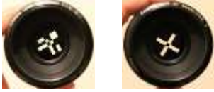
Fig. 5. Lens assembled with proposed masks.
