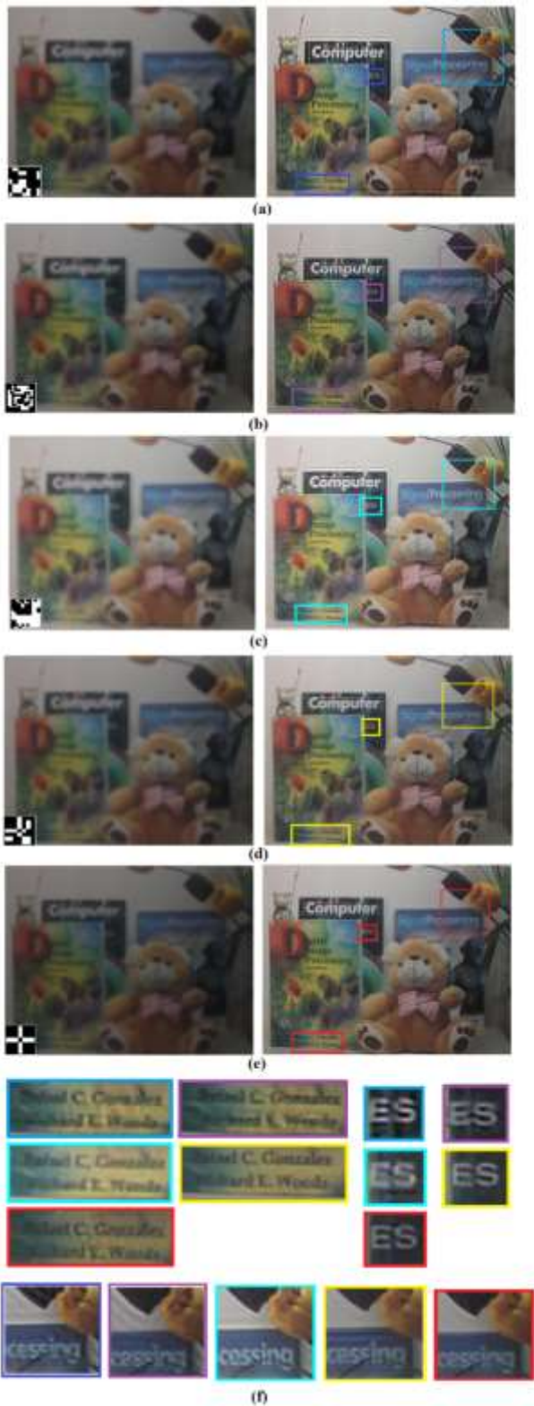
Fig. 9. Captured image and deblurred result in depth 80cm for five different apertures (a) Veeraraghavan[3], (b) Zhou[2], (c) Masia[4], (d) Asymmetric and (e) semi-symmetric patterns. (f) Close-ups of deblurred images.
